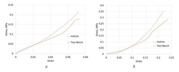
Fig. 3. Typical "stress-strain" dependences obtained on a testing machine and a mobile test bench: a -for hard plaques; b -for soft plaques
