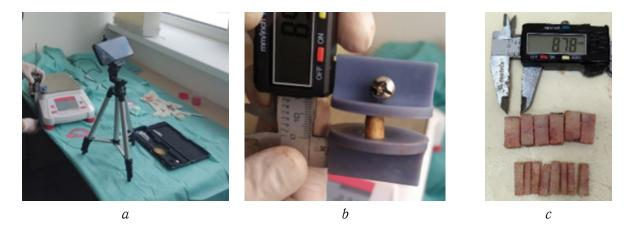
Fig. 1. The test bench components and typical samples: a is the general view; b are special removable platforms for caliper and a cylindrical sample of the plaque; c are samples of bovine cancellous bone (color online)
